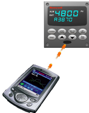
Figure 1-3 Depiction of infrared communications
