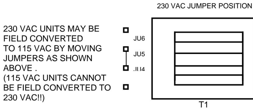
FIGURE A-2 - Processor Board
