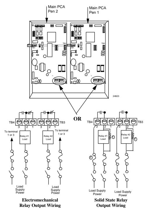
① If the load current is less than the minimum rated value of 20 mA, there may be a residual voltage across both ends of the load even if the relay is turned off. Use a dummy resistor as shown to counteract this. The total current through the resistor and the load current must exceed 20 mA.
