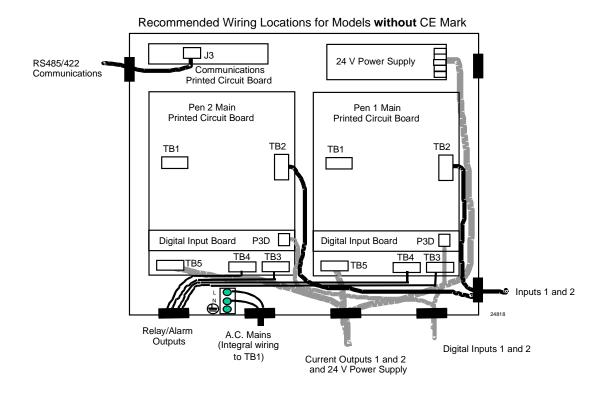
Figure 2-7 Recommended Wiring Routing - Models Without CE Mark
