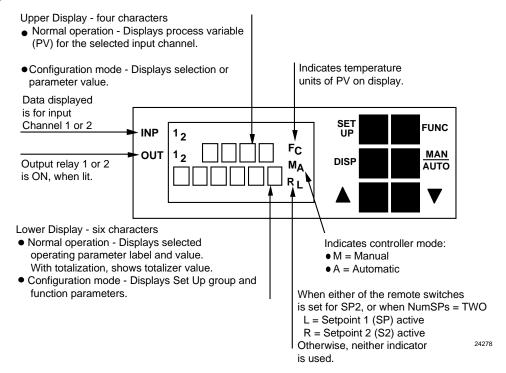
Figure 4-7 Operator Interface
