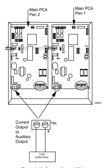
Figure 2-16 Current Output Wiring
