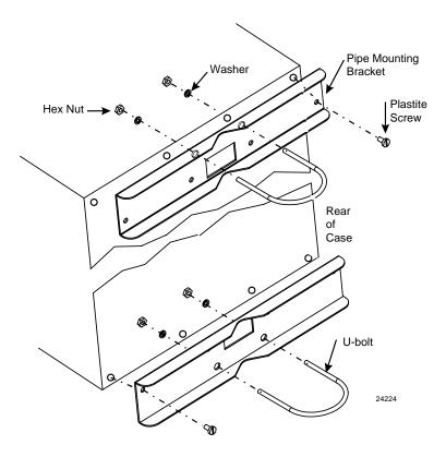
Figure 2-5 Pipe Mounting Brackets
