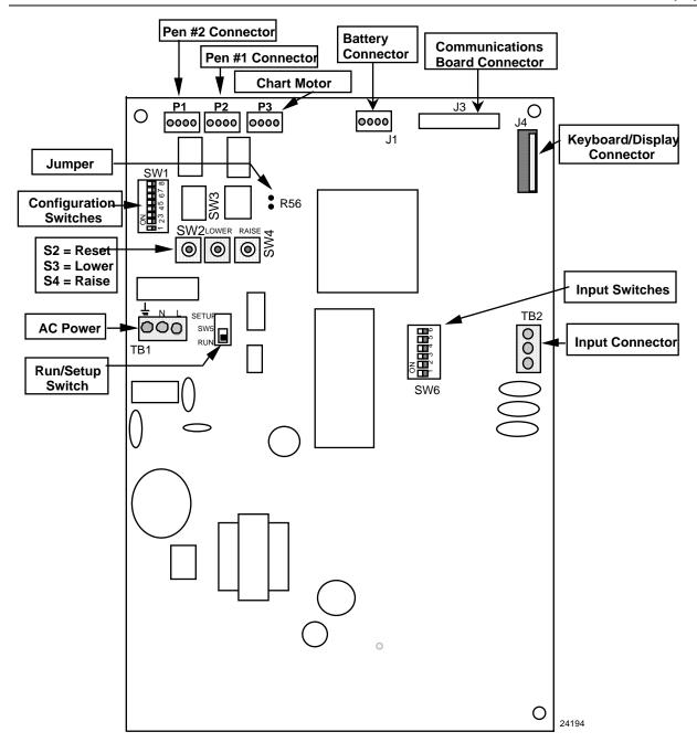
Figure 3-1 Location of Configuration and Input Switches
