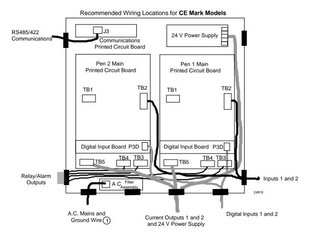
1 A braided copper shield shall be connected to ground (green screw on the filter assembly).
