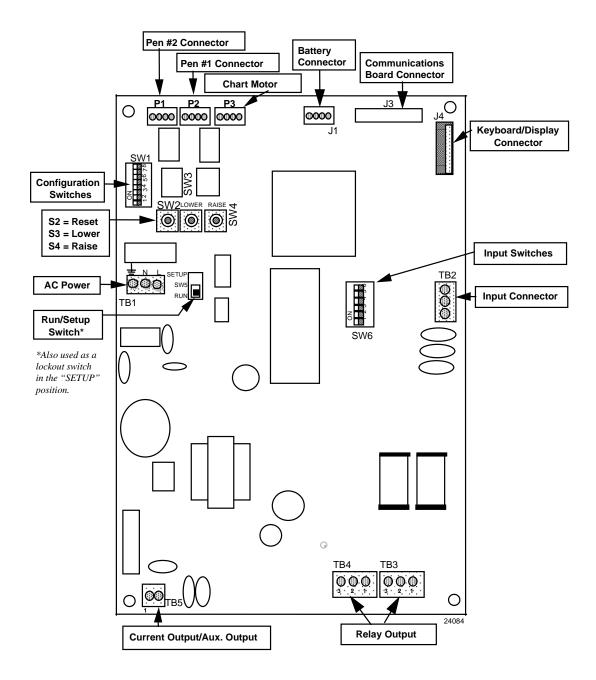
Figure 4-3 Location of Switches and Relays
