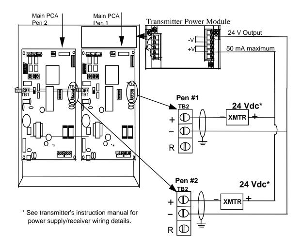
Figure 2-17 Transmitter Power Out Wiring
