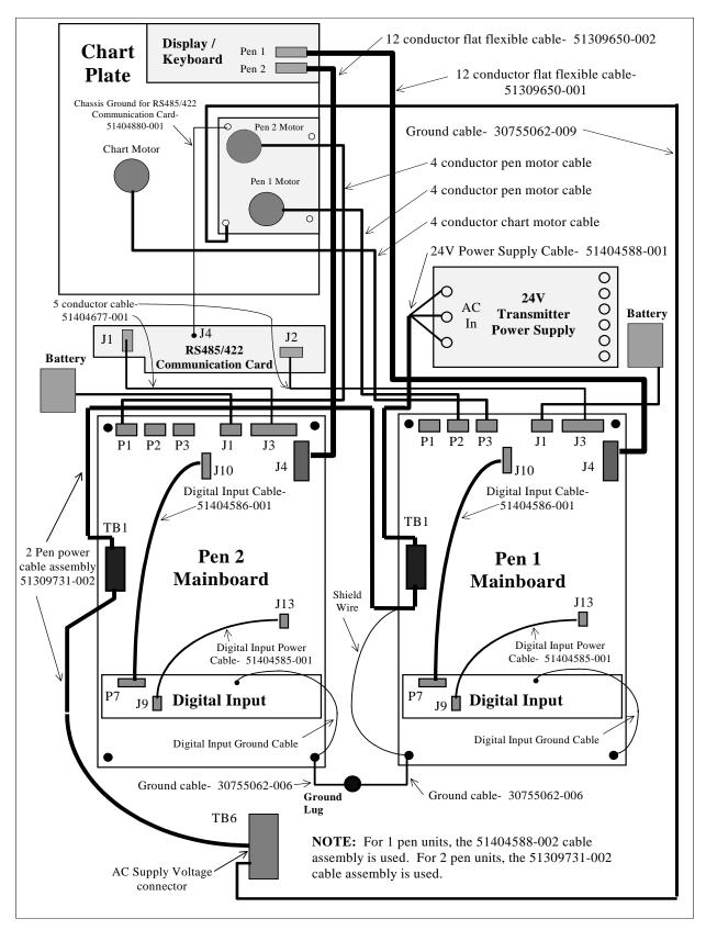
Figure 9-5 DR4300 Recorder (Non-CE Mark) – Internal Cabling Diagram
