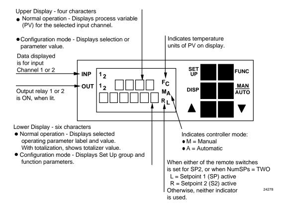
Figure 4-1 Operator Interface
