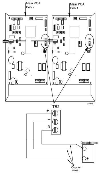
Figure 5-4 Calibration Set Up Diagram for RTD Inputs
