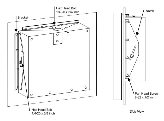
NOTE: Mounting brackets and attaching hardware are included in kit 30755065-502; panel gasket supplied in kit 51197657-501.
