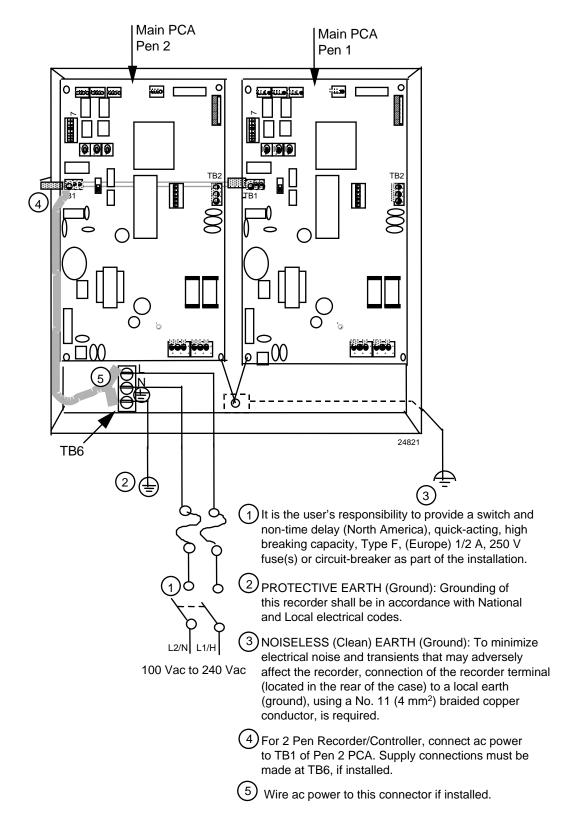
Figure 2-9 Power Wiring – Models Without CE Mark
