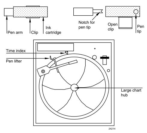
Figure 6-1 Replacing the Chart and Ink Cartridge
