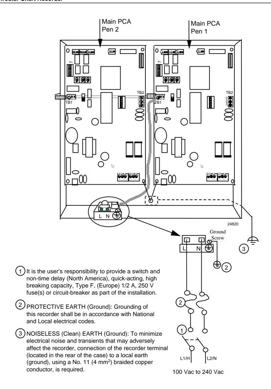
Figure 2-10 Power Wiring – Models With CE Mark
