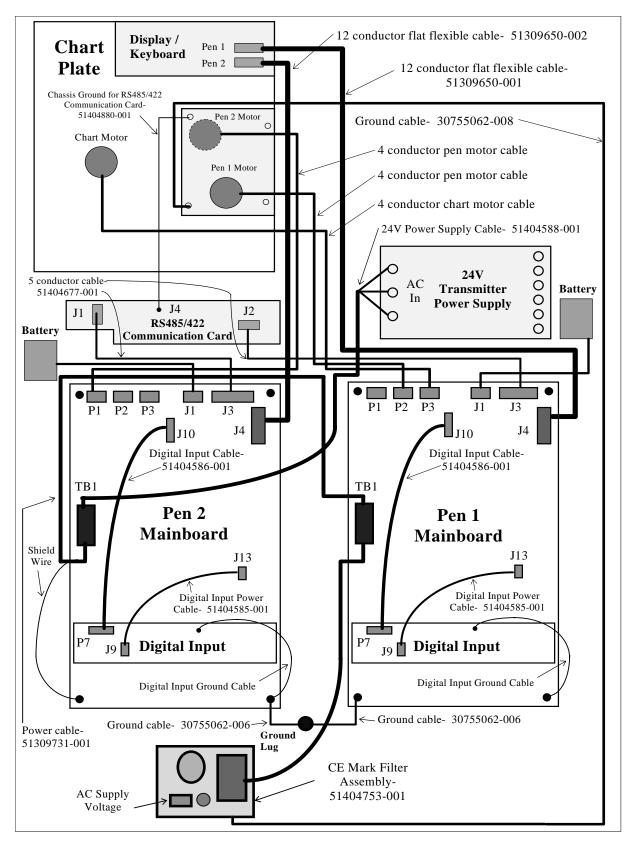
Figure 9-4 DR4300 Recorder (CE Mark) - Internal Cabling Diagram
