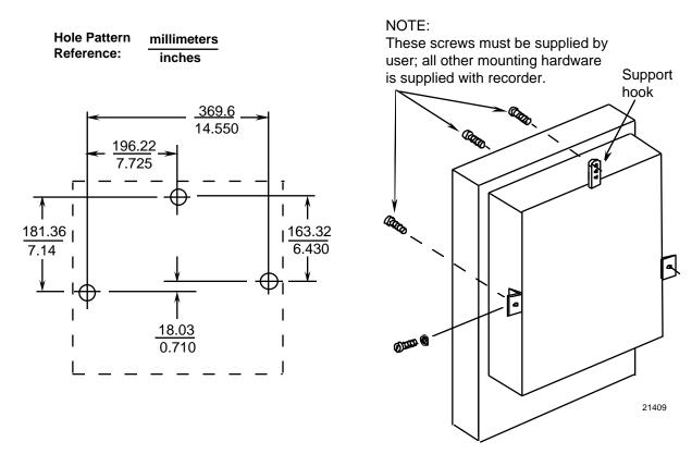
Figure 2-6 Mounting Flush on a Surface of Panel or Wall (Rear View)
