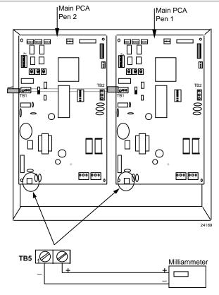
Figure 5-6 Test Equipment Connections for Calibrating Current Output
