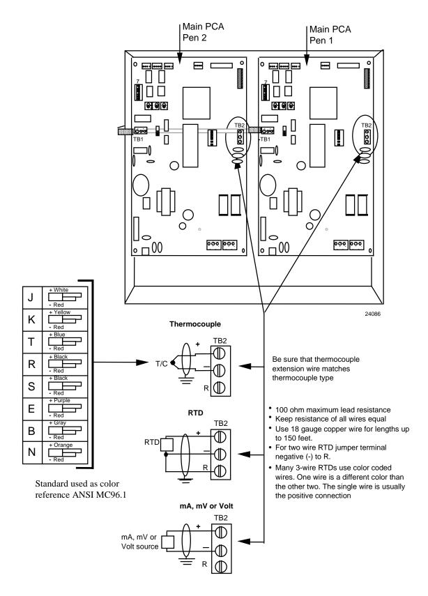
Figure 2-11 Analog Input Wiring
