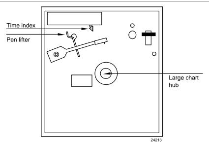
Figure 3-3 Basic Chart Plate Components
