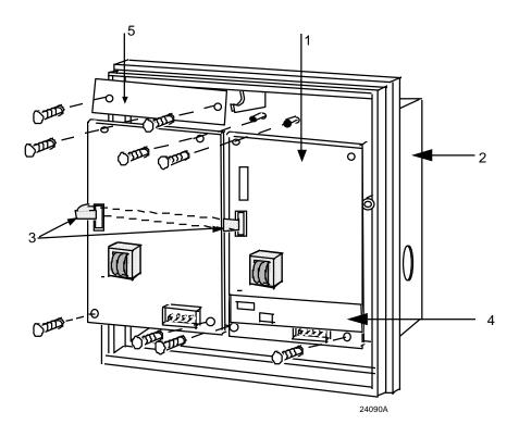
Figure 9-3 Recorder Components
