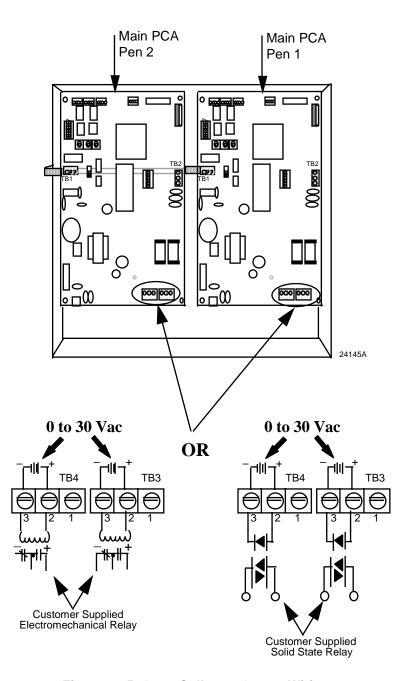
Figure 2-15 Open Collector Output Wiring
