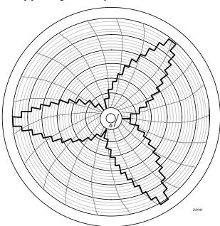
Figure 4-5 Typical Step Test Chart Patterns
